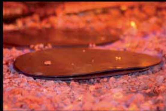
Discs are heated in a wood fired oven..
