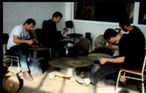
Hand hammering to create the shape..
